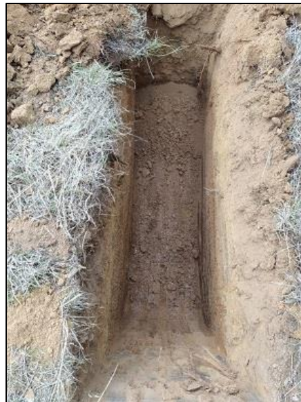
Plate 8: Shallow refusal on hardpan ferricrete horizon
