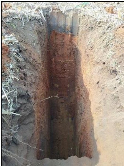
Plate 7: Typical residual siltstone soils extending to between 2.5 and 3m before grading into siltstone bedrock
