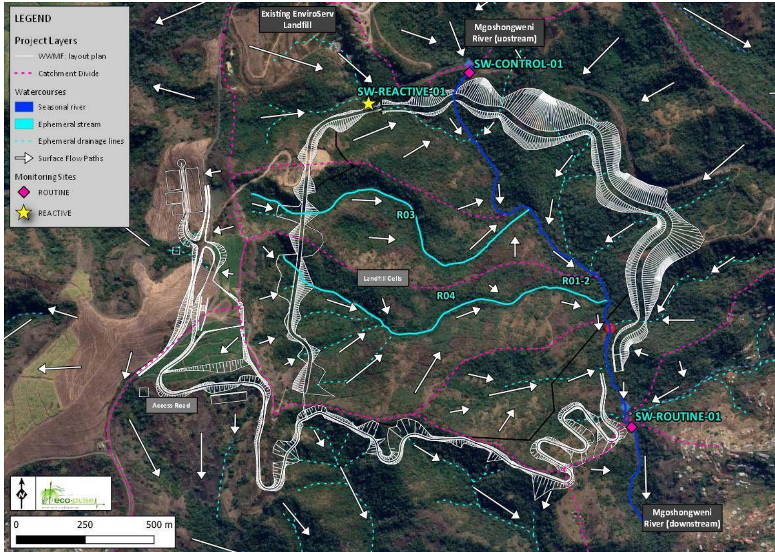
Figure 28 Map showing the location of (i) Routine and (ii) Reactive water quality and aquatic biomonitoring sites in relation to rivers and streams on the development property and downstream.
