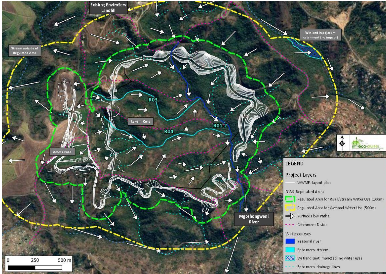
Figure 14 Map showing the location of identified and delineated watercourses: rivers and streams relative to the planned landfill development layout.
